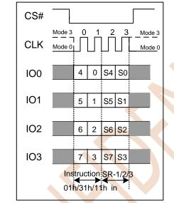
Figure 7.5b Write Status Register Instruction(QPI Mode)
