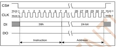
Figure 7.37a Individual Block/Sector Unlock Instruction(SPI Mode)
