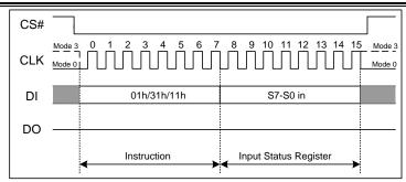
Figure 7.5a Write Status Register Instruction(SPI Mode)
