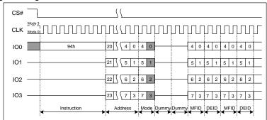
Figure 7.42 Read Manufacturer/Device ID Quad I/O Instruction
