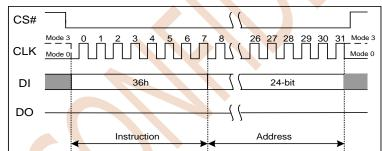
Figure 7.36a Individual Block/Sector Lock Instruction(SPI Mode)
