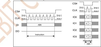
Figure 7.28 Release Power-down Instruction(SPI and QPI Mode)
