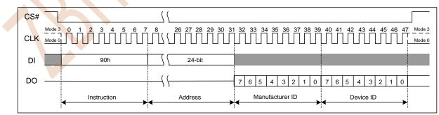
Figure 7.30a Read Manufacturer/Device ID(SPI Mode)
