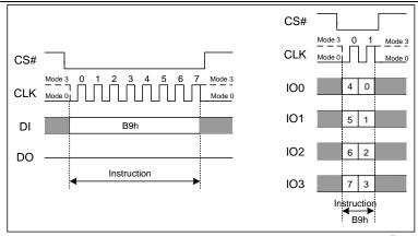
Figure 7.27 Deep Power-down Instruction(SPI and QPI Mode)
