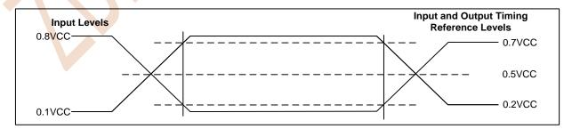
Figure 8.3 AC Measurement I/O Waveform
