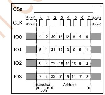
Figure 7.36b Individual Block/Sector Lock Instruction(QPI Mode)
