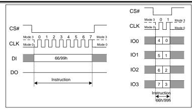
Figure 7.26 Software Reset Instruction(SPI and QPI Mode)
