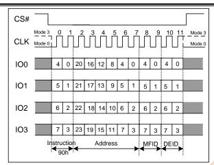
Figure 7.30b Read Manufacturer/Device ID(QPI Mode)
