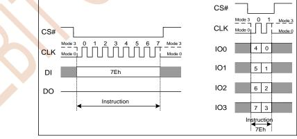
Figure 7.39 Global Block Lock Instruction(SPI or QPI Mode)
