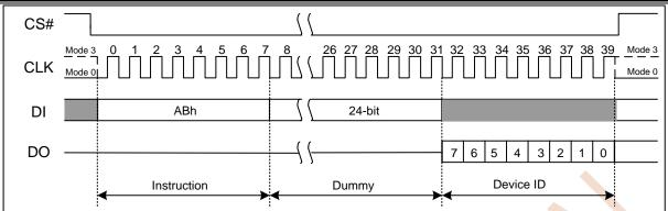
Figure 7.25 Release Power-down / Device ID
