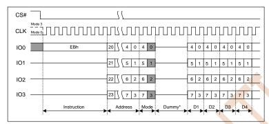
Figure 7.19 Fast Read Quad I/O Instruction(Initial command or previous M5-4 ≠10)
