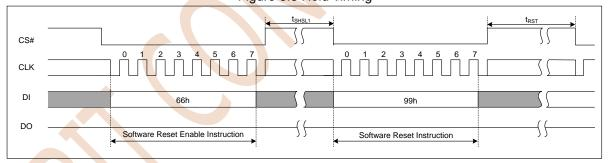
Figure 8.7 Software Reset Input Timing
