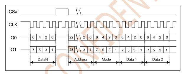
Figure 7.18 Fast Read Dual I/O Instruction (Initial command or previous M5-4=10)
