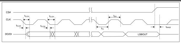
Figure 8.4 Serial Output Timing
