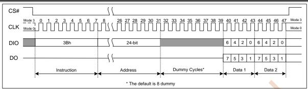
Figure 7.11 Fast Read Dual Output Instruction Sequence Diagram
