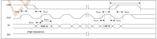
Figure 8.5 Input Timing
