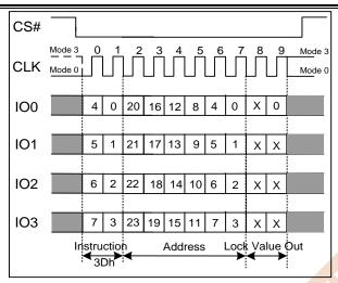
Figure 7.42b Read Block Lock Instruction(QPI Mode)
