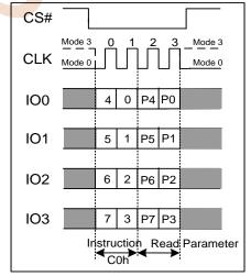
Figure 7.37 Set Read Parameters Instruction (QPI Mode only)
