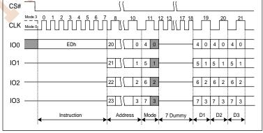
Figure 7.21a DTR Fast Read Quad I/O Instruction (M7-0 = FFh, SPI Mode)
