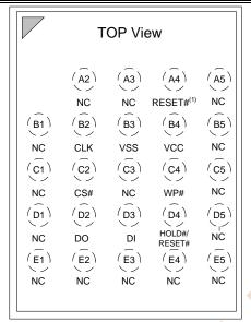
Figure 3.4 24-BALL TFBGA (5x5 ball array)
