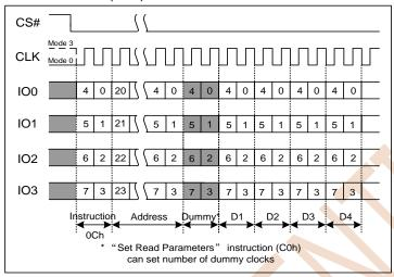
Figure 7.38 Burst Read with Wrap Instruction (QPI Mode only)
