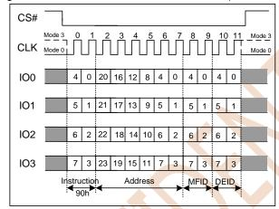
Figure 7.28b Read Manufacturer/Device ID(QPI Mode)
