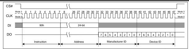
Figure 7.28a Read Manufacturer/Device ID(SPI Mode)
