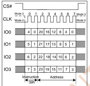
Figure 7.41a Individual Block/Sector Unlock Instruction(SPI Mode)
