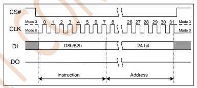
Figure 7.9a Block Erase Instruction(SPI Mode)
