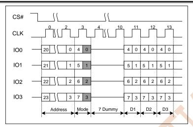
Figure 7.21b DTR Fast Read Quad I/O Instruction(Previous command set M5-4 = 10)
