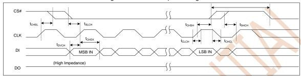
Figure 8.5 Input Timing
