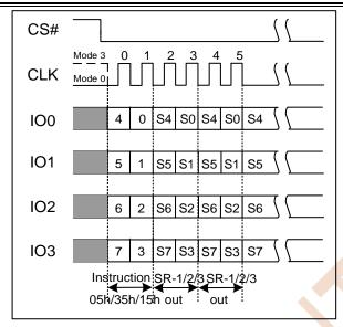
Figure 7.1b Read Status Register Instruction(QPI Mode)
