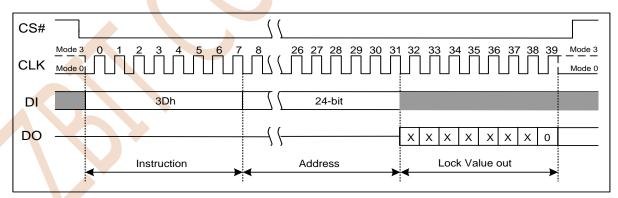
Figure 7.42a Read Block Lock Instruction(SPI Mode)
