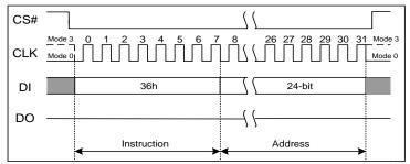
Figure 7.40a Individual Block/Sector Lock Instruction(SPI Mode)
