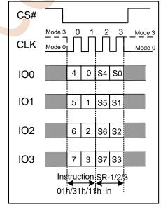
Figure 7.5b Write Status Register Instruction(QPI Mode)
