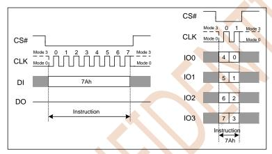
Figure 7.12 Erase/Program Resume Instruction(SPI or QPI Mode)
