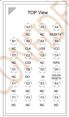
Figure 3.5 24-BALL TFBGA (6x4 ball array)
