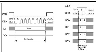
Figure 7.44 Global Block Lock Instruction(SPI or QPI Mode)
