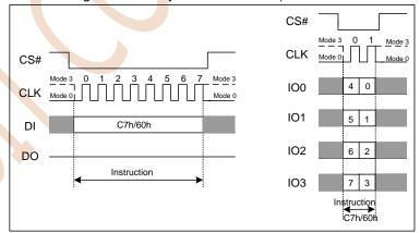
Figure 7.10 Chip Erase Instruction(SPI or QPI Mode)
