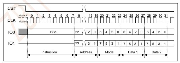
Figure 7.18a Fast Read Dual I/O Instruction (Initial command or previous M5-4≠10)
