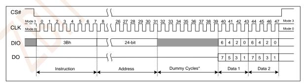
Figure 7.16 Fast Read Dual Output Instruction Sequence Diagram
