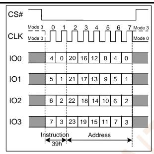
Figure 7.41b Individual Block/Sector Unlock Instruction(QPI Mode)
