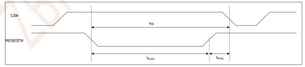
Figure 8.8 Hardware Reset Timing
