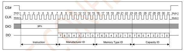
Figure 7.29a Read JEDEC ID(SPI Mode)
