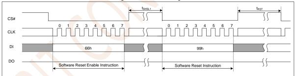
Figure 8.7 Software Reset Input Timing
