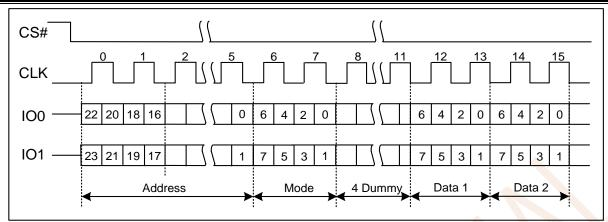
Figure 7.19b DTR Fast Read Dual I/O Instruction (Previous M5-4=10, SPI Mode only)
