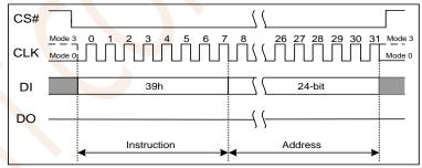
Figure 7.41 Individual Block/Sector Unlock Instruction(SPI Mode)
