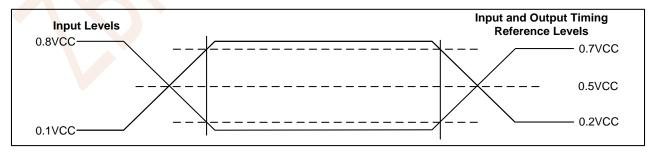
Figure 8.3 AC Measurement I/O Waveform
