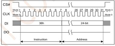
Figure 7.40a Individual Block/Sector Lock Instruction(SPI Mode)
