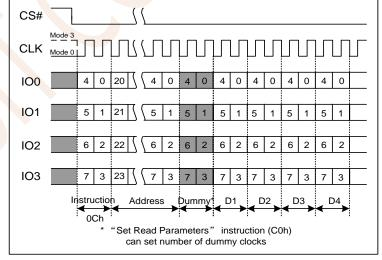
Figure 7.38 Burst Read with Wrap Instruction (QPI Mode only)
