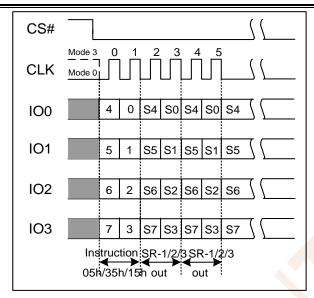
Figure 7.1b Read Status Register Instruction(QPI Mode)
