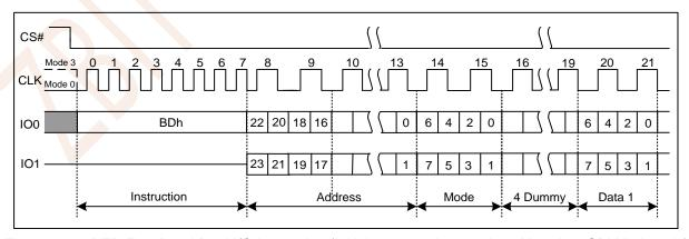
Figure 7.19a DTR Fast Read Dual I/O Instruction (Initial command or previous M5-4≠10, SPI Mode only)
