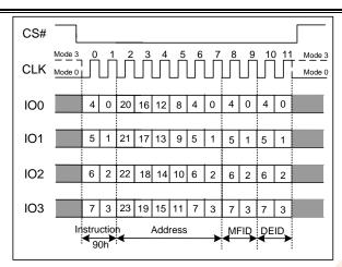
Figure 7.28b Read Manufacturer/Device ID(QPI Mode)
