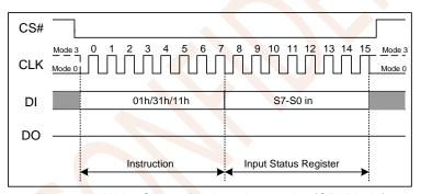
Figure 7.5 Write Status Register Instruction(SPI Mode)
