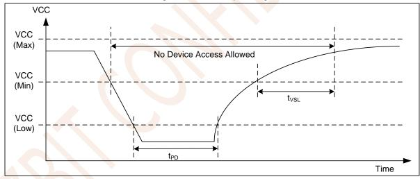
Figure 8.2 Power-Down and Voltage Drop
