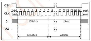
Figure 7.9a Block Erase Instruction(SPI Mode)
