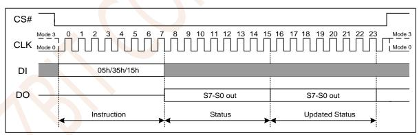
Figure 7.1a Read Status Register Instruction(SPI Mode)
