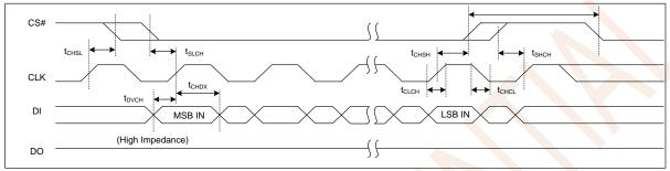
Figure 8.5 Input Timing
