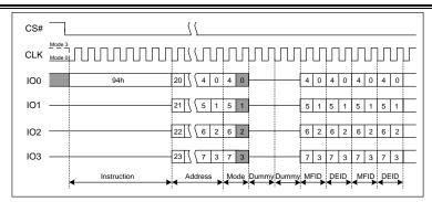
Figure 7.35 Read Manufacturer/Device ID Quad I/O Instruction
