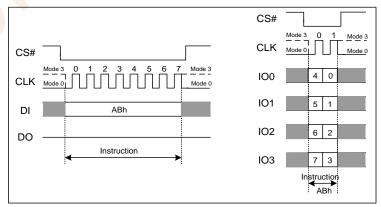
Figure 7.26 Release Power-down Instruction(SPI and QPI Mode)
