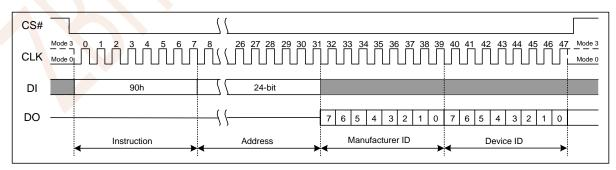
Figure 7.28a Read Manufacturer/Device ID(SPI Mode)
