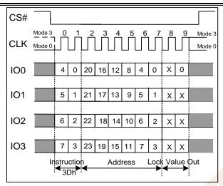
Figure 7.42b Read Block Lock Instruction(QPI Mode)
