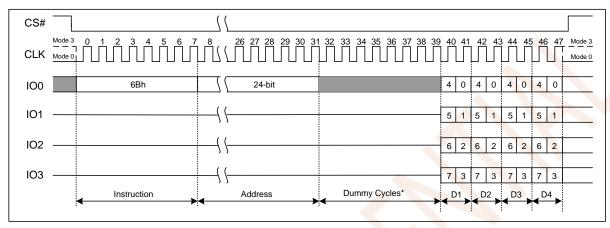
Figure 7.17 Fast Read Quad Output Instruction
