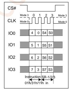
Figure 7.5b Write Status Register Instruction(QPI Mode)
