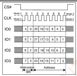
Figure 7.40b Individual Block/Sector Lock Instruction(QPI Mode)
