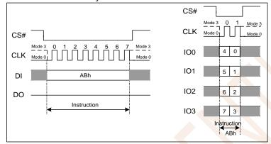
Figure 7.27 Release Power-down Instruction(SPI and QPI Mode)
