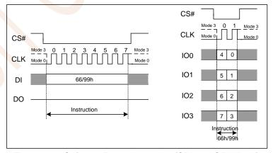
Figure 7.25 Software Reset Instruction(SPI and QPI Mode)
