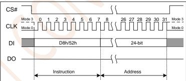
Figure 7.9a Block Erase Instruction(SPI Mode)
