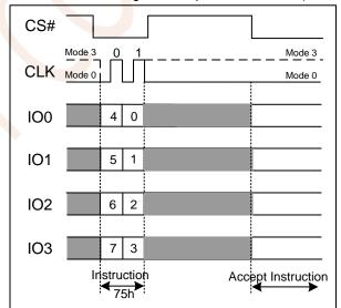
Figure 7.11b Erase / Program Suspend Instruction(QPI Mode)
