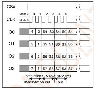
Figure 7.1b Read Status Register Instruction(QPI Mode)
