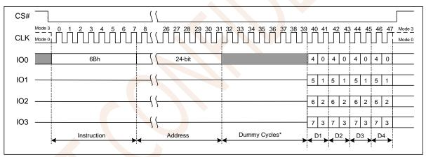
Figure 7.16 Fast Read Quad Output Instruction
