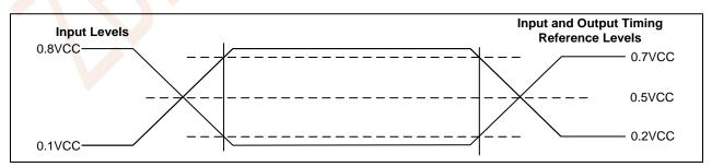
Figure 8.3 AC Measurement I/O Waveform
