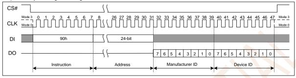
Figure 7.30a Read Manufacturer/Device ID(SPI Mode)
