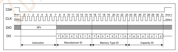
Figure 7.31a Read JEDEC ID(SPI Mode)
