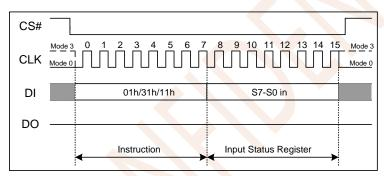
Figure 7.5a Write Status Register Instruction(SPI Mode)
