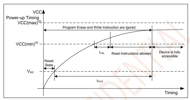
Figure 8.1 Power-up Timing
