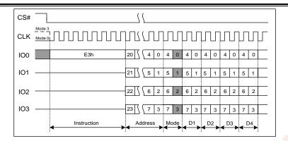
Figure 7.22 Octal Word Read Quad I/O Instruction(Initial command or previous M5-4 ≠10)
