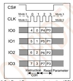
Figure 7.39 Set Read Parameters Instruction (QPI Mode only)
