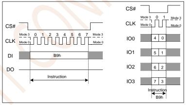
Figure 7.26 Deep Power-down Instruction (SPI and QPI Mode)
