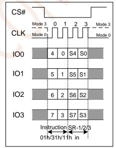
Figure 7.5b Write Status Register Instruction(QPI Mode)
