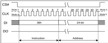
Figure 7.36 Read Manufacturer/Device ID Dual I/O Instruction
