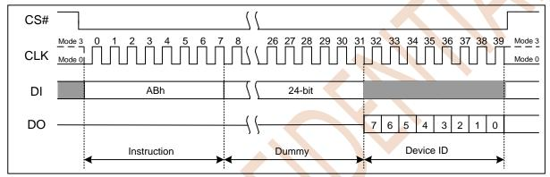
Figure 7.14 Release Power-down / Device ID
