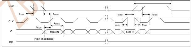
Figure 8.5 Input Timing
