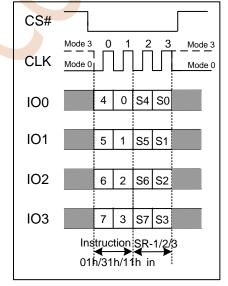
Figure 7.5b Write Status Register Instruction(QPI Mode)
