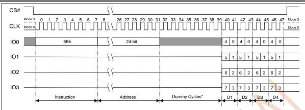
Figure 7.16 Fast Read Quad Output Instruction
