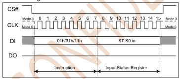
Figure 7.5a Write Status Register Instruction(SPI Mode)
