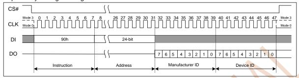
Figure 7.30a Read Manufacturer/Device ID(SPI Mode)
