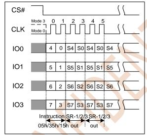
Figure 7.1b Read Status Register Instruction(QPI Mode)
