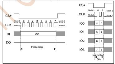
Figure 7.2 Write Enable Instruction(SPI or QPI Mode)
