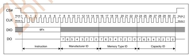
Figure 7.31a Read JEDEC ID(SPI Mode)
