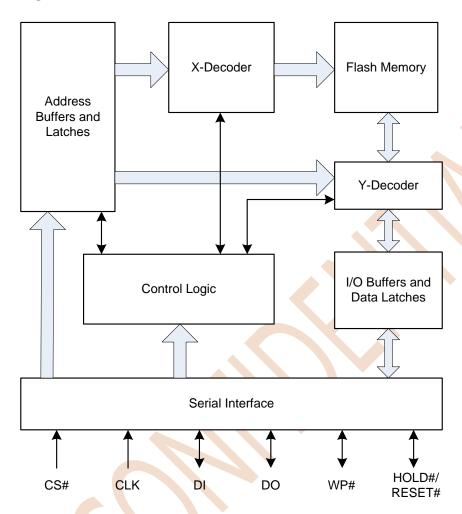
Figure 2.1 Block Diagram
