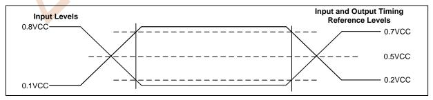
Figure 8.3 AC Measurement I/O Waveform
