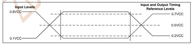
Figure 8.3 AC Measurement I/O Waveform
