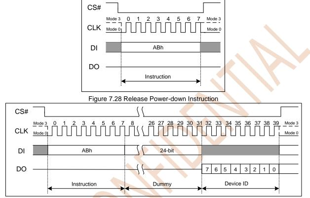
Figure 7.29 Release Power-down / Device ID
