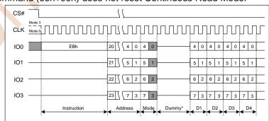
Software reset command (66h+99h) does not reset Continuous Read Mode.
