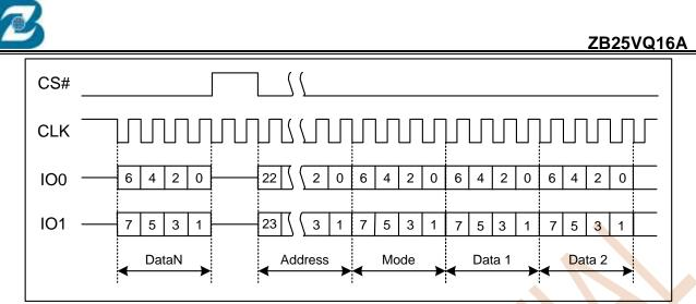
Figure 7.18 Fast Read Dual I/O Instruction (Initial command or previous M5-4=10)
