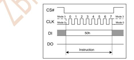
Figure 7.3 Write Enable for Volatile Status Register Instruction
