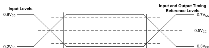
Figure 8.3 AC Measurement I/O Waveform
