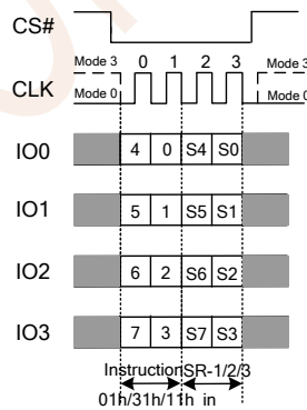
Figure 7.5b Write Status Register Instruction(QPI Mode)
